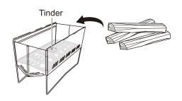
The definition of "fuel" in this user's manual means logs, sticks and charcoal. Dry twigs, sticks and bark are suitable for tinder. Wood from broad-leafed trees makes excellent material for fires as it burns hotter and longer. The Folding Fire Pit is designed to accommodate fuel with a maximum length of 40 cm, while the Folding Fire Pit S is designed to accommodate fuel with a maximum length of 30 cm.
